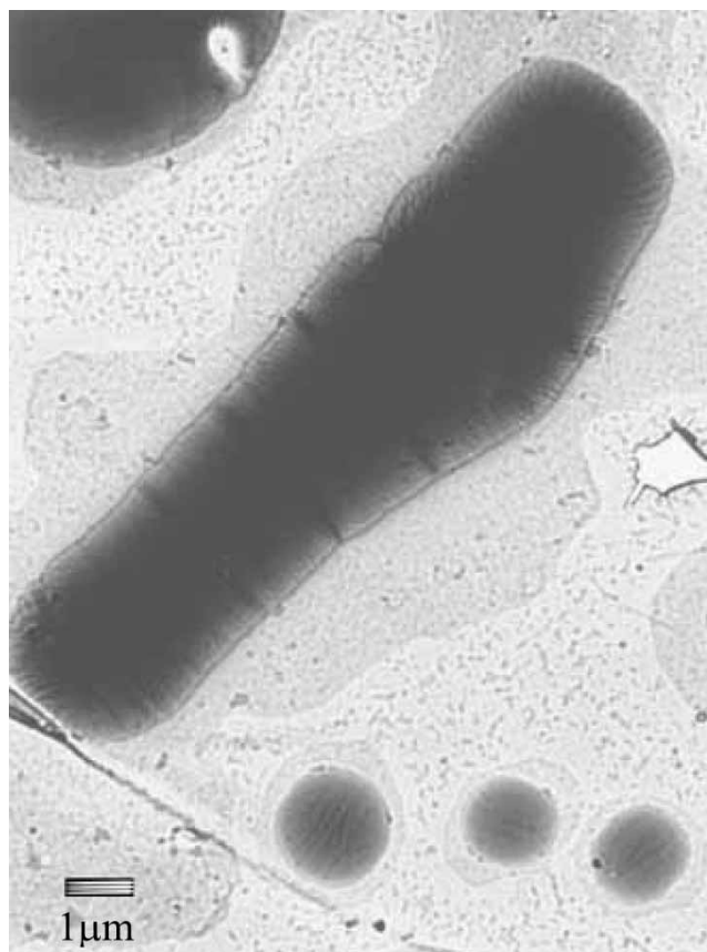
Figure 10. TEM morphology of PA9EO7 imaged with electron beam parallel to the layer planes of the smectic B phase.
